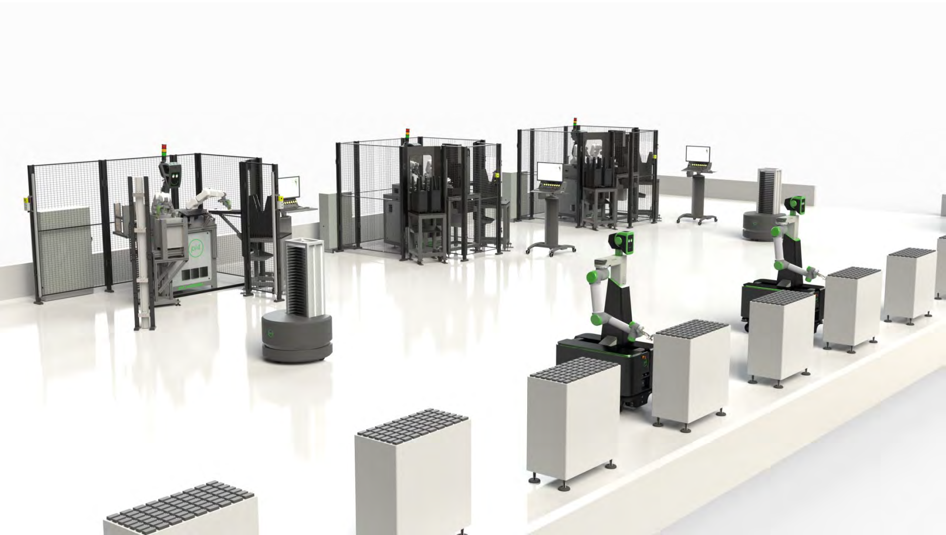
Workerbot6-M loading / unloading jobs e.g. electronic testing
