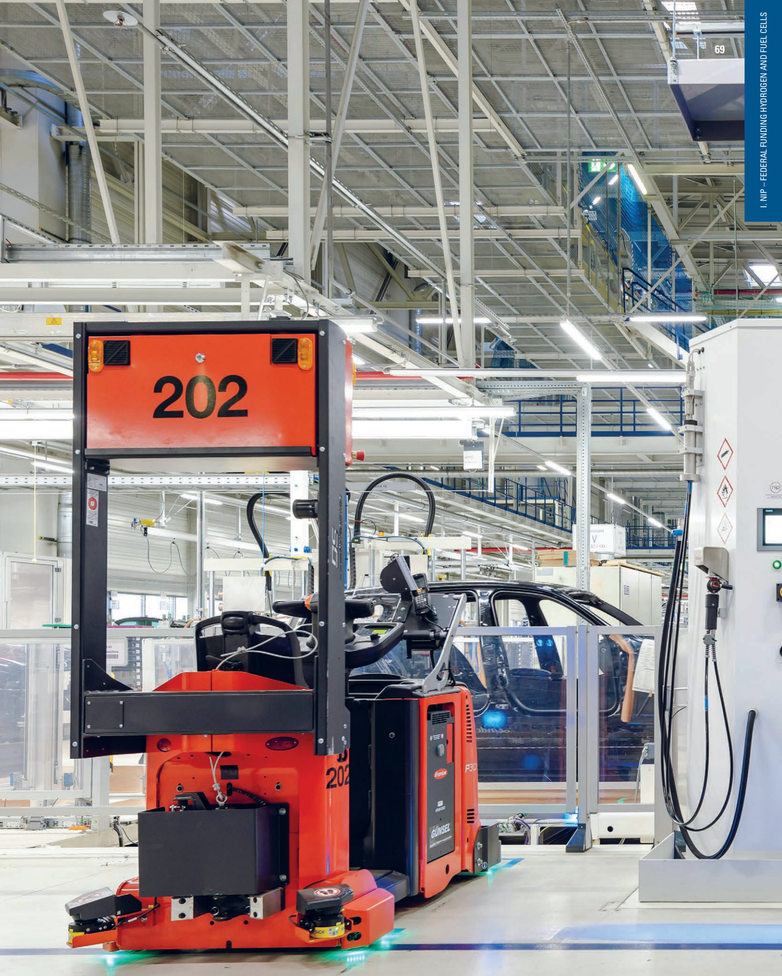
Fuel cells in use: At the BMW plant in Leipzig, 70 hydrogen-powered tugger trains (indoor tugs) from Linde Material Handling are responsible for intralogistics.
