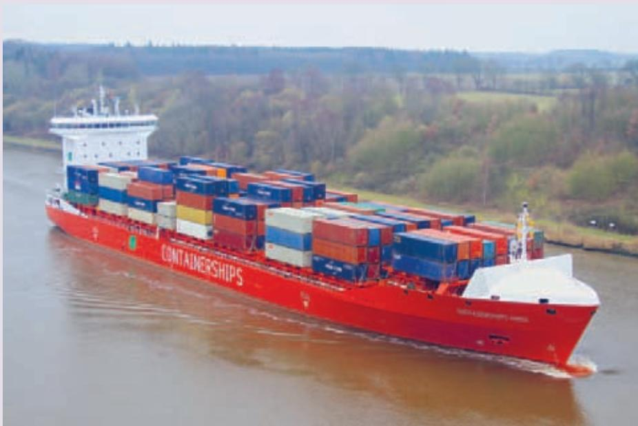
The already operating MV 'Containerships Nord', very similar to the subsidised ships, is a 1,400 TEU dual fuel container ship, owned by the Nordic Hamburg shipping company.
