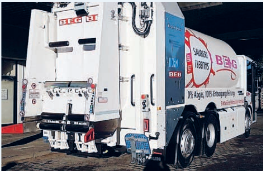
Zero emission fuel cell-based waste collection vehicle
