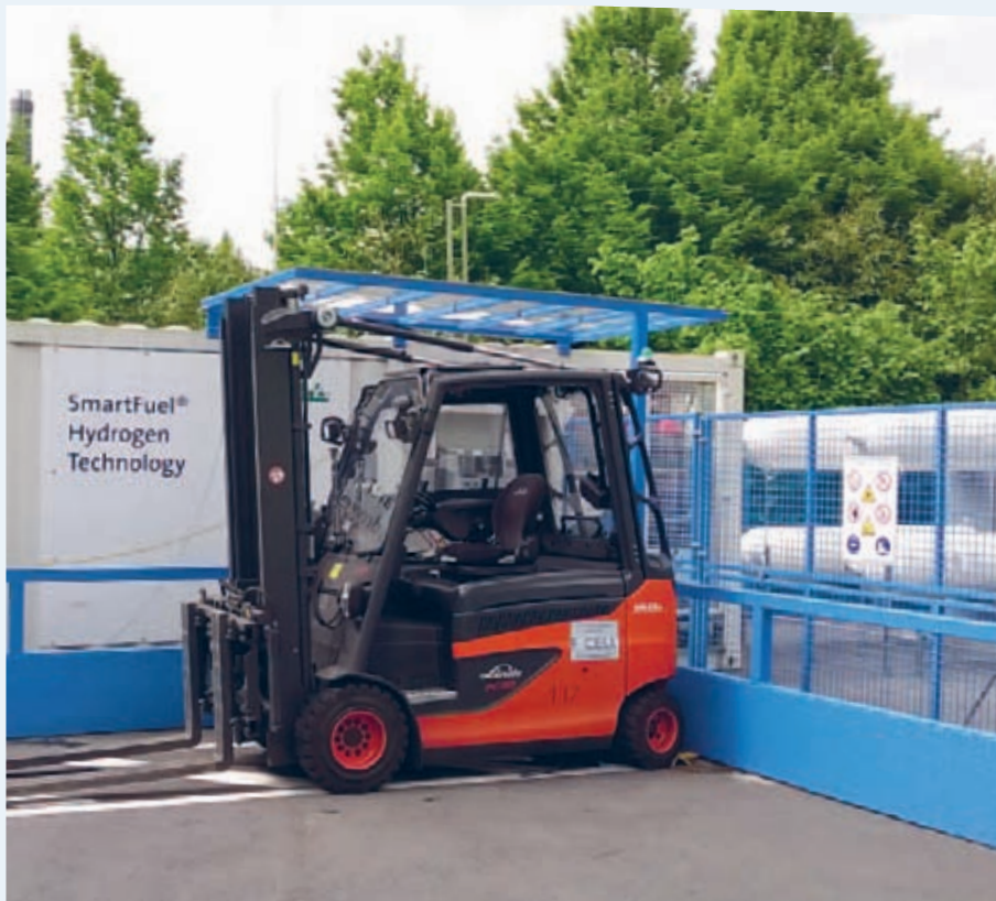
Forklift with fuel cell drive used for on-site logistics transport
