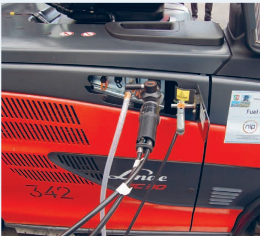
Refuelling a materials handling vehicle with hydrogen
