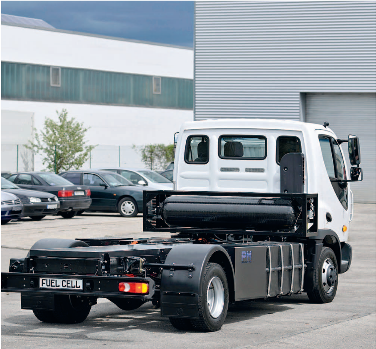
Vehicle chassis with integrated range extender system
