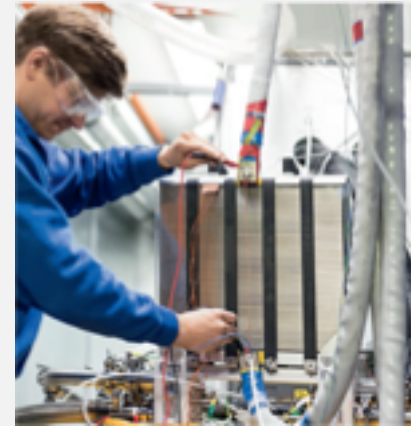
Automotive FC-Stack 100 kW (©: ZSW)
