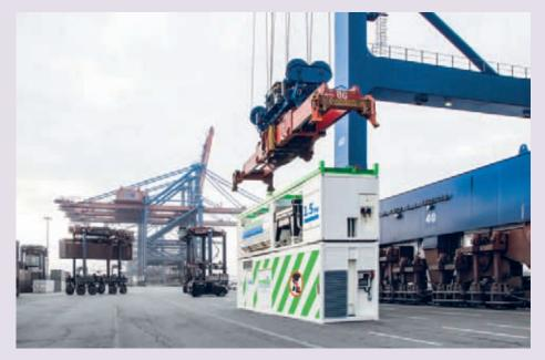
The prototype of the LNG PowerPac, a mobile containerised solution for shore-side power supply, undergoes a 24-hour test operation at the Burchardkai container terminal in the Port of Hamburg in June 2019.
