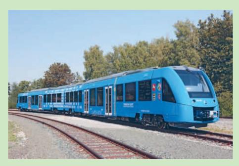
Since 2018, the regional public transport company of Lower Saxony (LNGV – Landesnahverkehrsgesellschaft Niedersachsen) has deployed two Coradia iLint local trains with hydrogen fuel cell drives. In the first six months of operation in 2019, the trains covered 100,000 km: quietly, without emissions and reliably.
