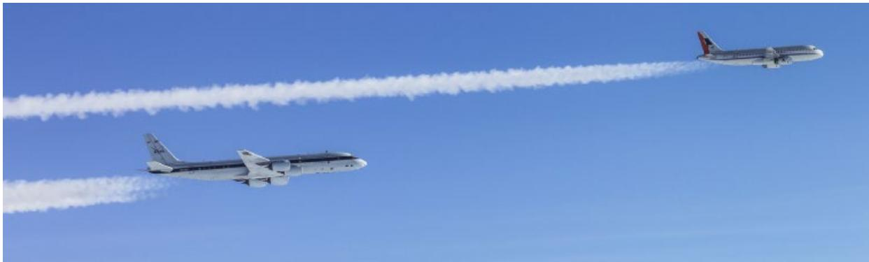
The NASA DC8 research aircraft probing contrails from the DLR A320 burning sustainable aviation fuel blends. Photo showing the DC8 chasing a contrail from the A320 burning a sustainable aviation fuel blend above Germany on 24 January 2018.<sup>1</sup>
