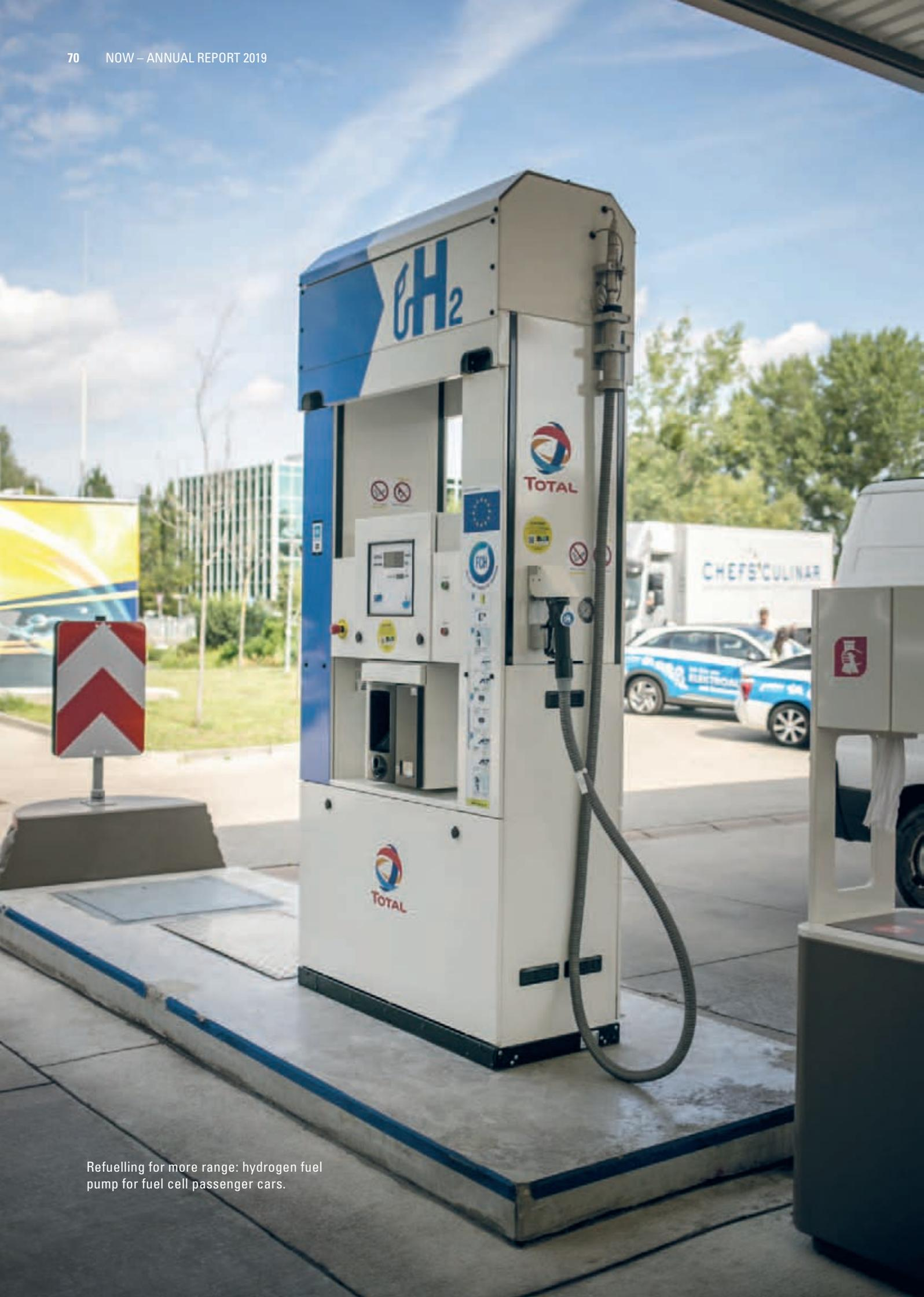
Refuelling for more range: hydrogen fuel pump for fuel cell passenger cars.
