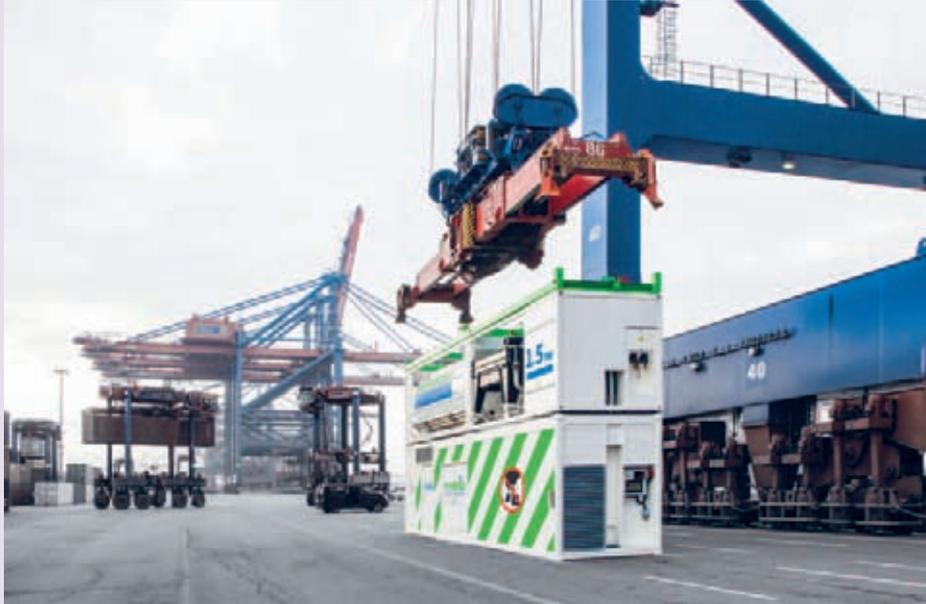
The prototype of the LNG PowerPac, a mobile containerised solution for shore-side power supply, undergoes a 24-hour test operation at the Burchardkai container terminal in the Port of Hamburg in June 2019.
