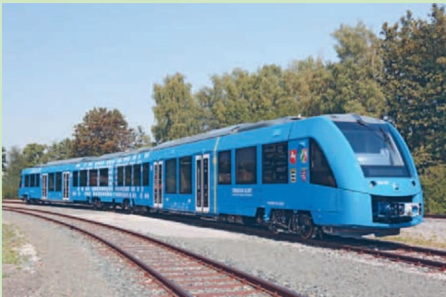
Since 2018, the regional public transport company of Lower Saxony (LNGV – Landesnahverkehrsgesellschaft Niedersachsen) has deployed two Coradia iLint local trains with hydrogen fuel cell drives. In the first six months of operation in 2019, the trains covered 100,000 km: quietly, without emissions and reliably.
