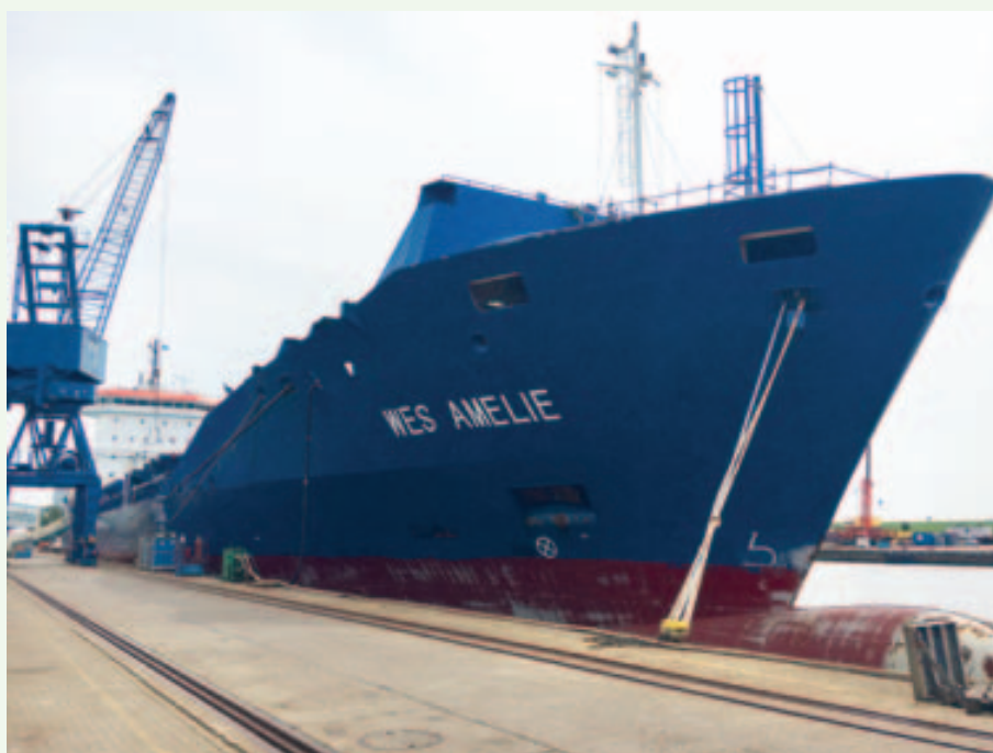
The world's first container ship converted to LNG: the Wes Amelie
