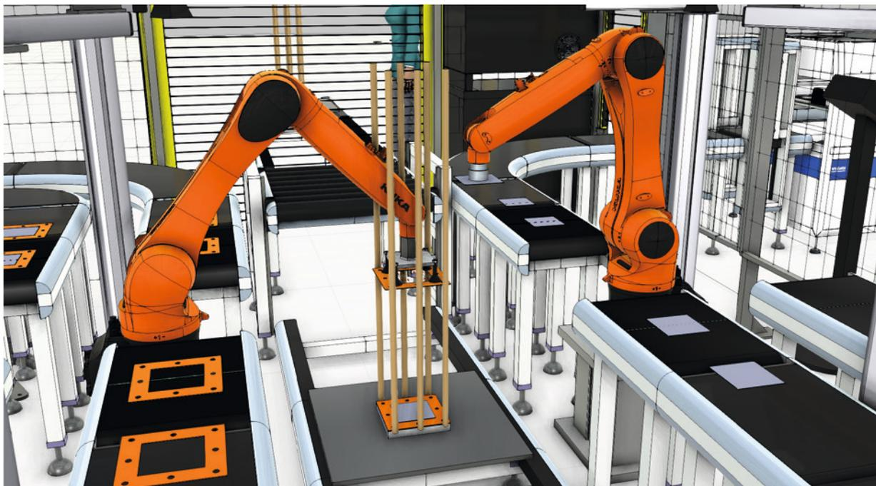
the preferable option, due to higher flexibility, lower cost and higher system availability. The deposition of the seven components per HT-cell then takes place directly on the lower end plate of the stack using two six-axis robots as shown in Figure 5-4.
